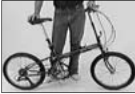
Getting ready for the quick fold. Release 2 quick release levers.
