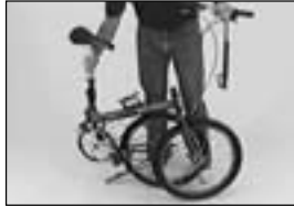
Remove the stem and fold down the seatmast.
